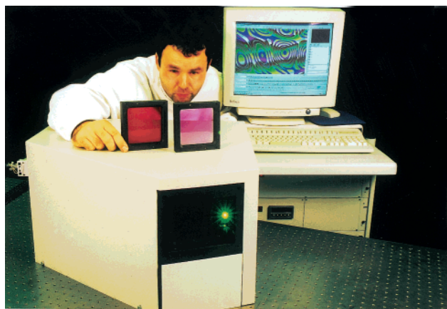
Figure 23. Prototype of a holographic camera for interferometric applications. All optical components are inside the camera head in the front. Bacteriorhodopsin films as they are used in the system are shown on top of the housing. In the rear the control unit can be seen. The operation of the system is completely under software control.
