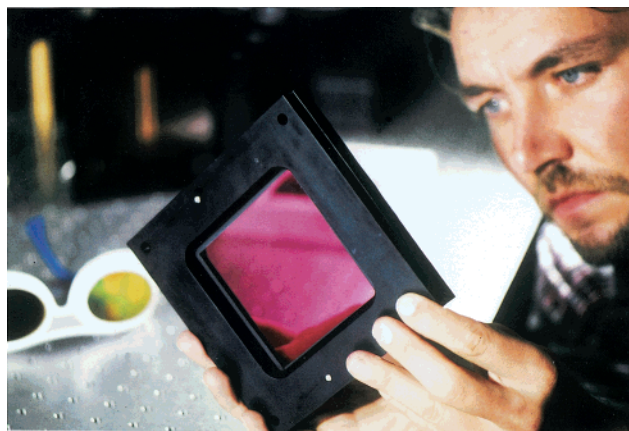
Figure 13. Bacteriorhodopsin film with large aperture. These films have free apertures of 90\text{ mm} \times 90\text{ mm} , their outer dimensions are 120\text{ mm} \times 120\text{ mm} . They are tuned to maximal light sensitivity because their primary use is in holographic interferometry.
